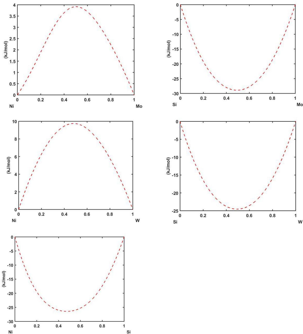
**Figure 1.** The formation enthalpy of the binary systems Ni-Pd, Si-Pd, Ni-Pt, Si-Pt, Ni-Zr, Si-Zr, Ni-Mo, Si-Mo, Ni-W, Si-W, and Ni-Si.
