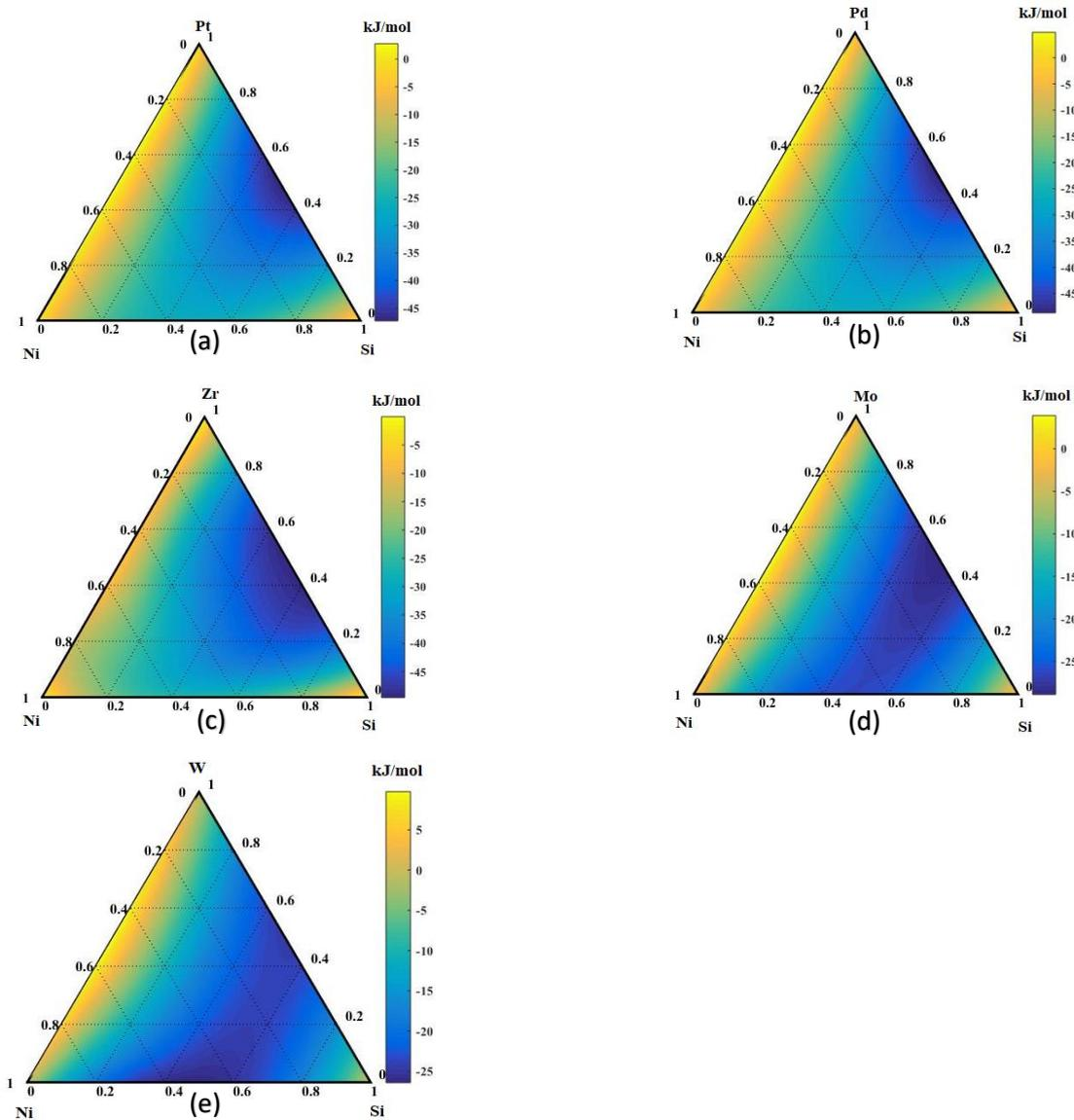
**Figure 2.** Formation enthalpy of ternary systems: (a) Ni-Pd-Si, (b) Ni-Pt-Si, (c) Ni-Zr-Si, (d) Ni-Mo-Si, and (e) Ni-W-Si.
