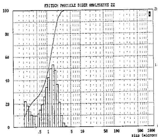
Figure 3. Particle size distribution of the milled powders.
