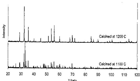
Figure 1. X-ray diffraction pattern of the calcined powders made by refined domestic iron oxide.
