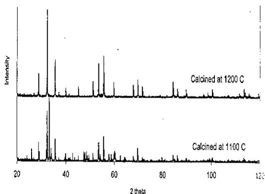
Figure 2. X-ray diffraction pattern of the calcined powders made by Merck iron oxide.
